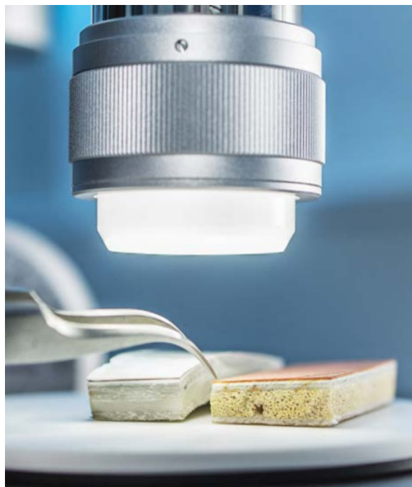
DFM provides reliable measurement technology that together with new drone-based technology will improve wind turbine owners' ability to monitor blade conditions. Wind-turbine blade section under the microscope.
