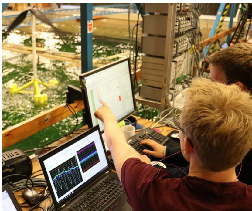
Danish businesses can use DHI's special wind turbine to test the performance of offshore structures such as floating windmills in severe wave and wind conditions.
